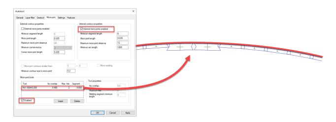
Outside arcs can have micro-joints when required by the *Maximum micro-joint* distance:
