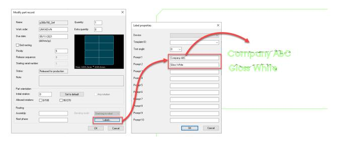
Normally the production label data comes from an order file (field ProductionLabel) through *Database* - *Orders*, similar to how label printers, inkjet and laser markers have been supported previously.
