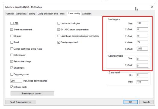
If M3P procedure fails the first measure, the machine updates the measure position increasing it by 25mm. Then it executes the measure again. This can cause collision because the new point can be inside the safe area.
