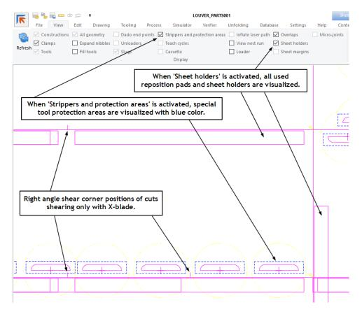
Positions of shear repositions (repositions made by using sheet holders of right angle shear) inside a zone are visualized with the right angle shear corner marker and an arrow, which length corresponds to the length of reposition. For repositions inside a zone, clamps and used reposition pads and sheet holders are visualized with a dashed line. For shear repositions between zones, used reposition pads and sheet holders are visualized with a solid line.
