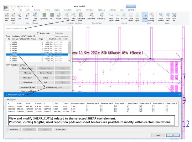
In new shearing NC syntax, all existing shearing commands are substituted with new commands. See comparison table below. '*Verifier*' supports the new NC syntax. Parameters of each SHEAR command can be seen in the Verifier visualizes used reposition pads and sheet holders with a darker color.
