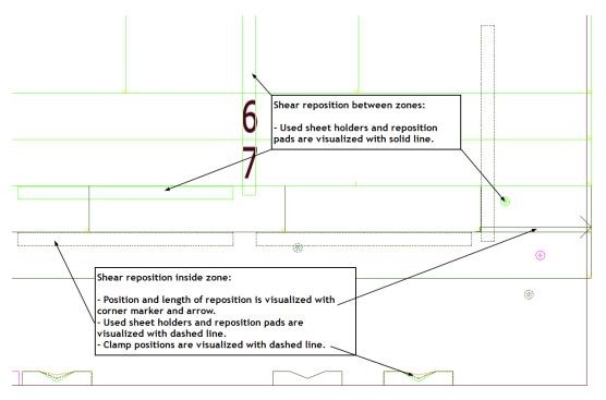
For cuts longer than X-blade of the shear, the optimizer divides the length of needed half-cuts (cuts shearing only with X-blade) evenly. Overlap of cuts in X-direction is minimized to prevent "hairs" which can occur when the same segment is cut twice.
