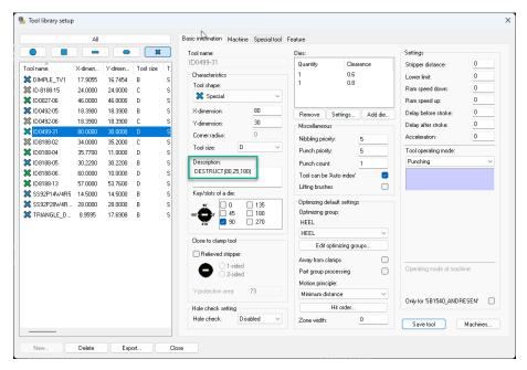
The tool is specially made for edge destructing, and it has the side support for punching narrow sheet edges for rather thick material. A normal rectangular tool will not last for long in this kind of use.
