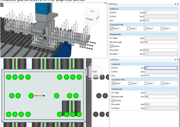
This functionality is automatically available in machines for which TulusParameters.xml has related options enabled. The USSPicking phase can be added by selecting it from BeltUnloadingSequence properties:
