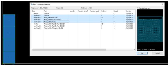
Parts are added inside the sheet when there is enough space and also to the *Part List* of the *Nesting parameters* dialog.
